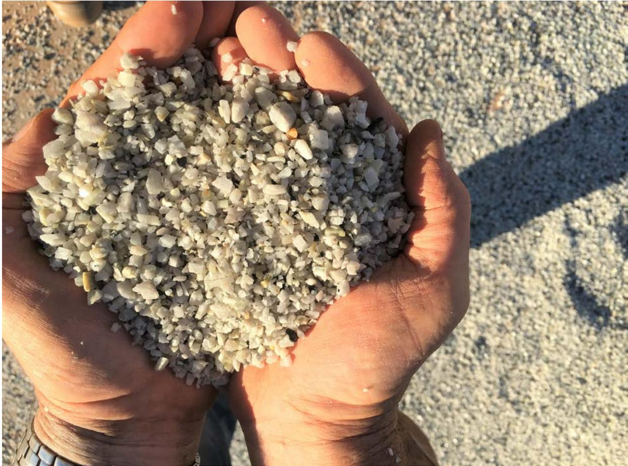
Figure 5 | Spodumene concentrate
